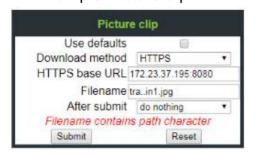
WBM checks that the file extension is valid for the type of file transfer
